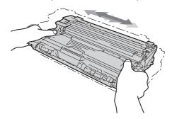
Slide all four drum and toner cartridge assemblies into the machine. Make sure the toner cartridge color matches the same color label on the machine.
